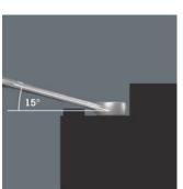
The ring side is tilted at 15° to the tool axis to prevent injury.
